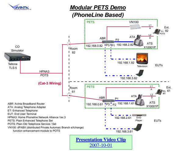
1. L1/A is an Analog dPABX over narrowband. The Extension number of each telephone station is set by rotary dials in VN100.
